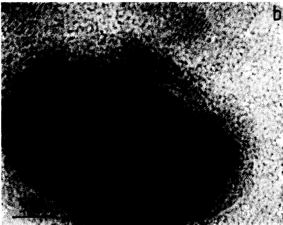
FIG. 8. (a) High-resolution image of small particle in the Ni Graphimet. The 70^\circ cross-grating pattern of 2.03\text{-}\text{\AA} lattice fringes identify the particle as being constituted of metallic Ni. (b) Partially overlapping particles showing 2.03\text{-}\text{\AA} Ni (111) lattice fringes in each, together with coarse spacing moiré fringes in the region of overlap.
