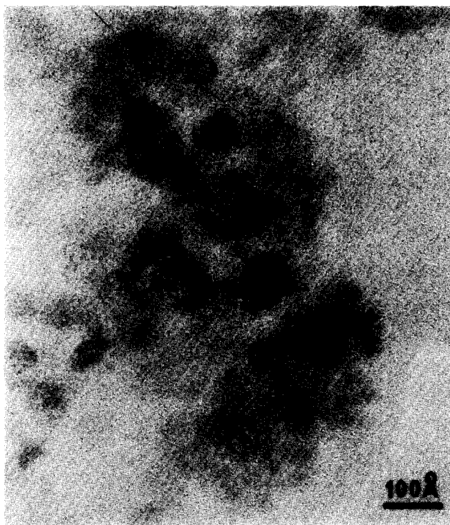
FIG. 5. Typical region of the Graphimet Co-5, showing clusters of \text{Co}_3\text{O}_4 particles supported by graphite.
